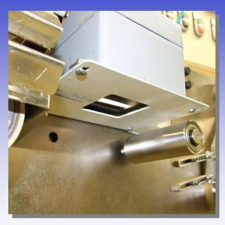
colour measurement of syntetic sausage casing
